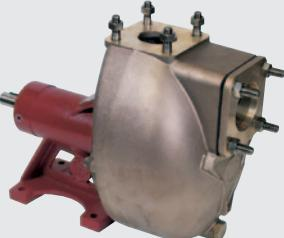
The AM pumps series are centrifugal self-priming with double volute body, the smaller size (DN 40-50) can be supplied for clockwise or anti-clock rotation and are characterized by high flow.
