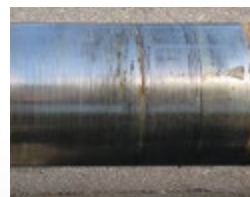
Shaft scoring caused by flax packing
