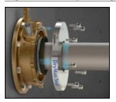
The DryMax™ primary sealing components can be renewed easily with the vessel at sea. With seawater restricted by the inflatable seal the split DuraChrome™ Mating Ring can be removed and the old seal ring replaced with the spare
