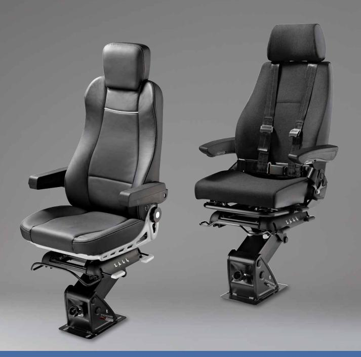
**OPERATOR PRO STAR** Special mission chair for naval and high-speed applications. A very special and strong shock-absorbing system combined with a proven mechanical suspension leads to ultimate power in »rough« seas and speedy operations. Also available with low backrest.
